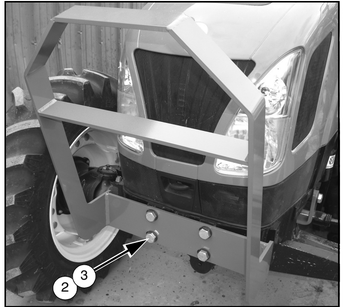
Figure 8. Grill Guard Installed
